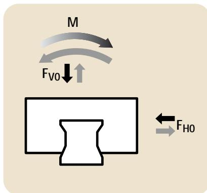
**Static equivalent bearing load**
